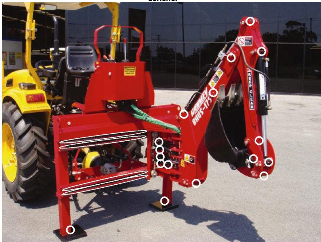
(Sliding bars for frame carrier require greasing Total of 19 grease nipples on BHUF & BHUS series Grease nipples are located on hver moving part) (gjelder ikke modellen du har kjøpt!)
